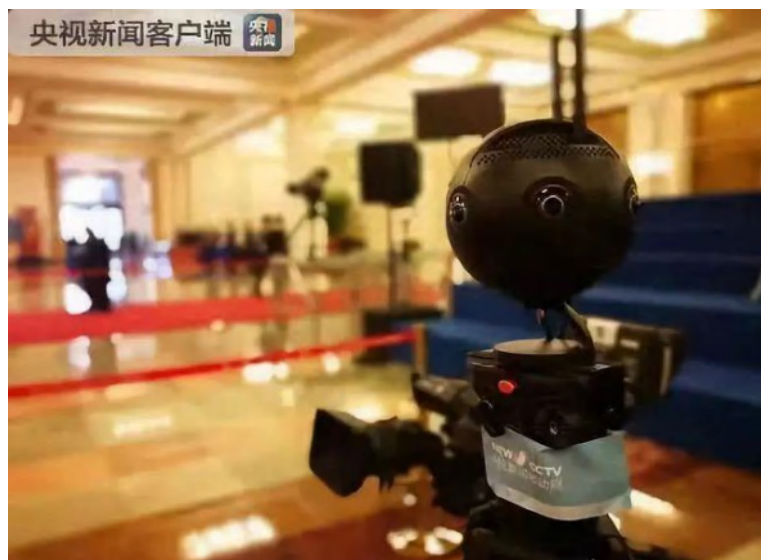
Figure 20 The “5G+4K” real-time backhaul (during the Two Sessions, China Media Group set up an outdoor camera on the top floor of the National Museum of China, and transferred 4K images in real time via China Unicom’s 5G network to the big screen.)
