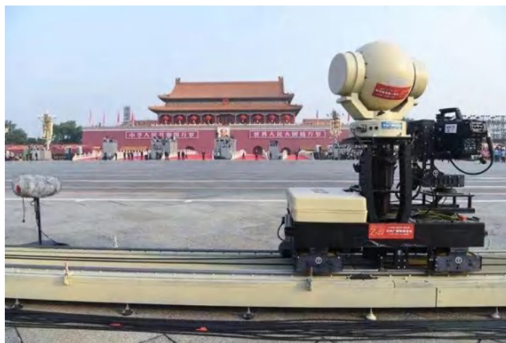
Figure 25 The 60-meter double-head electric track camera used by China Media Group in the live broadcasting of National Day events
